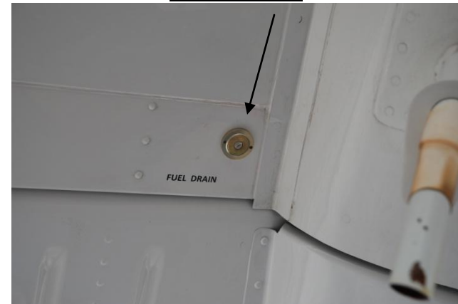
FIGURE 7-8 TANK SUMP DRAIN
