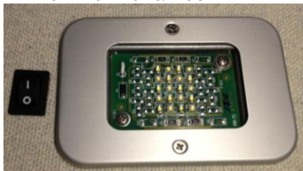
FIGURE 7-3 EMERGENCY CABIN LIGHTING SYSTEM CABIN SWITCH & FLOOD LAMP
