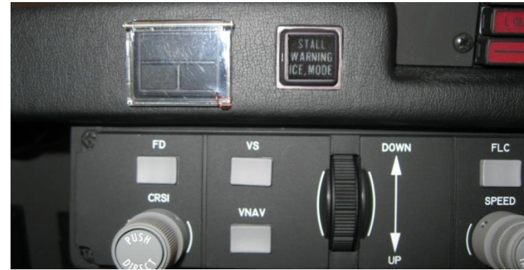
FIGURE 7-2 STALL WARNING ICE MODE ANNUNCIATOR
