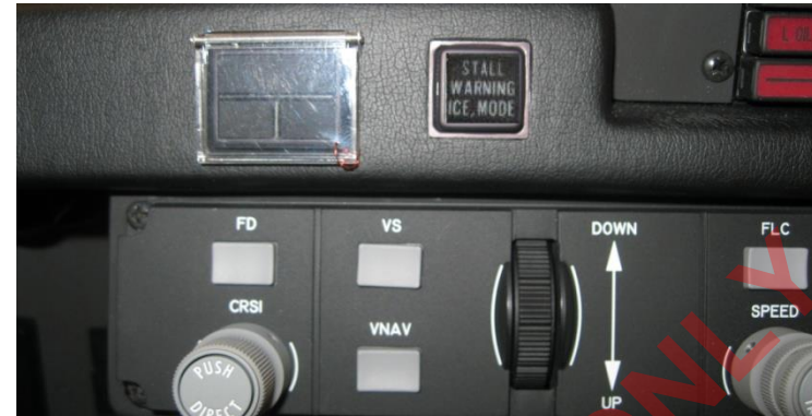
FIGURE 7-2 STALL WARNING ICE MODE ANNUNCIATOR
