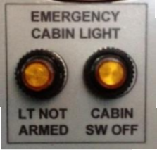
FIGURE 7-5 EMERGENCY CABIN LIGHTING SYSTEM WARNING LIGHTS
